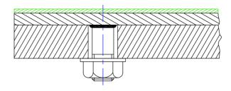
Welded-in Countersunk Insert [not recommended]
